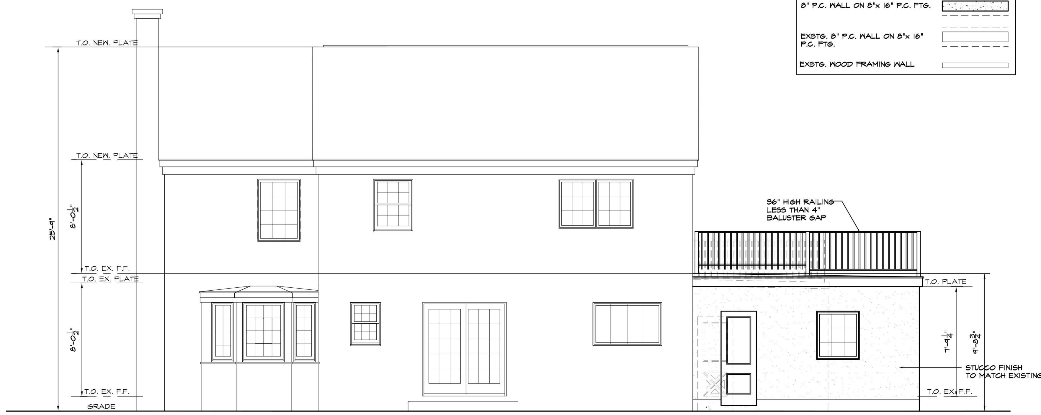
REAR ELEVATION SCALE 1/4" = 1'-0"
