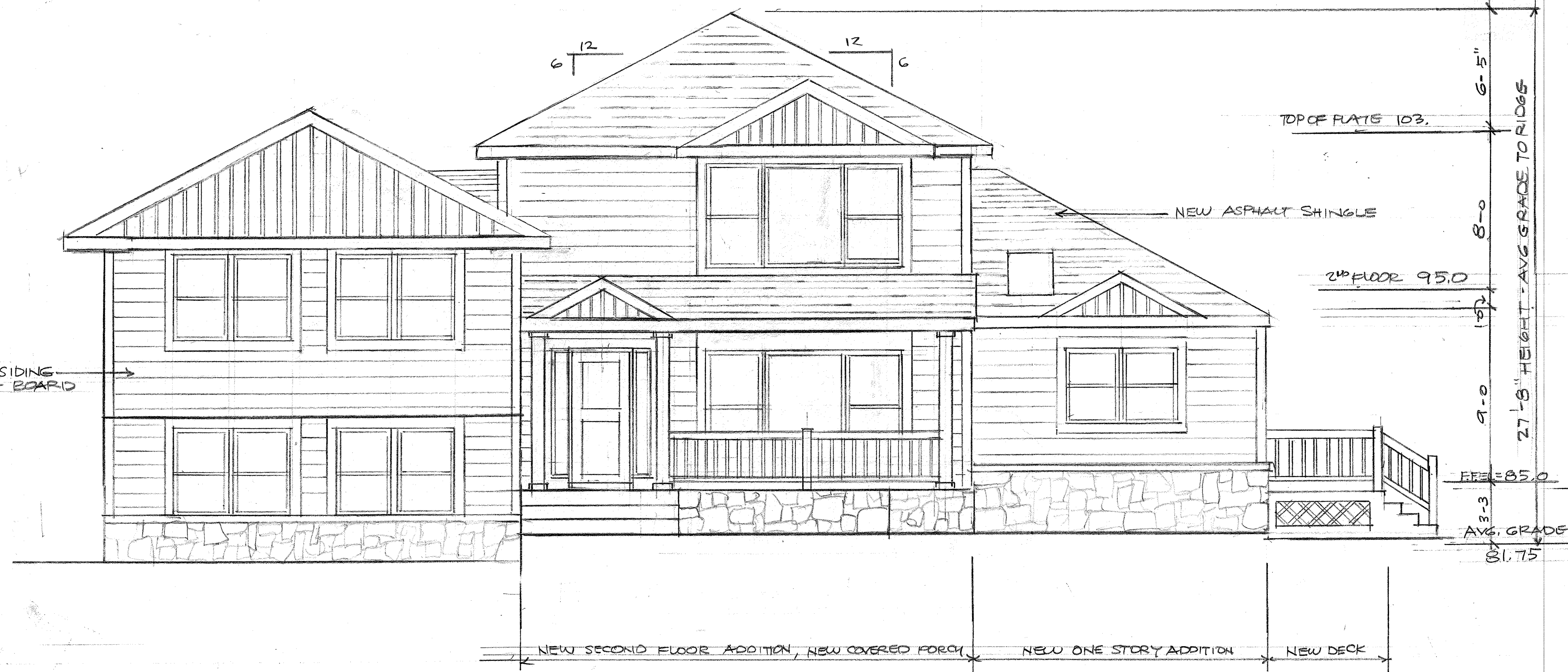
FRONT (EAST) ELEVATION 1/4"=1'-0"
