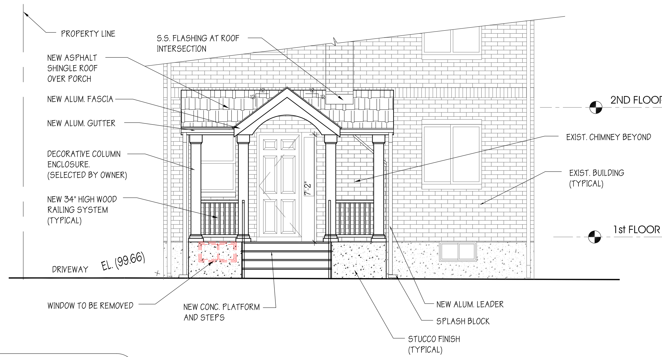
Porch Front Elevation
