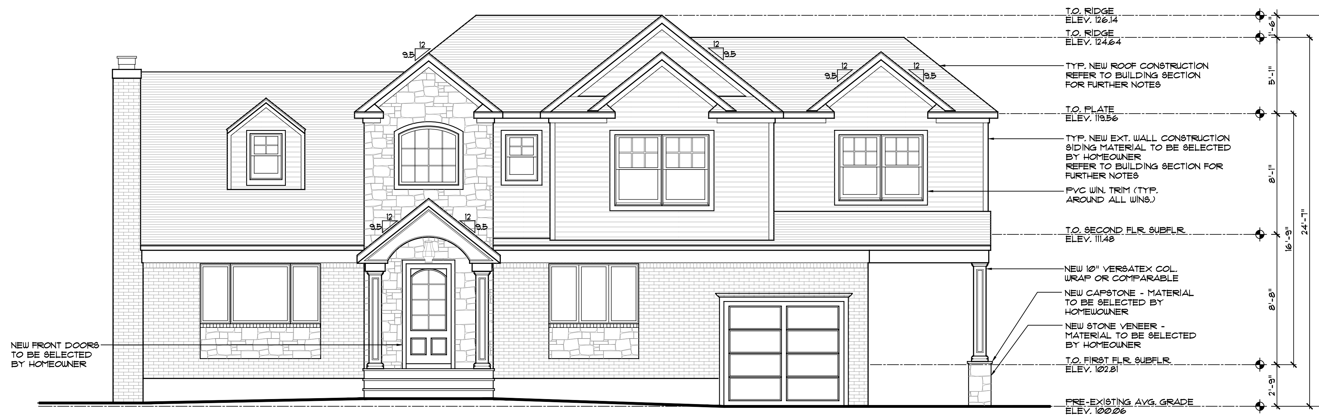
1 PROPOSED FRONT ELEVATION A-3 SCALE : 1/4" = 1'-0"
